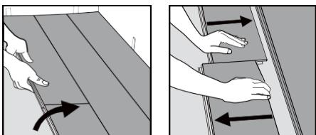
Separate the entire row by lifting it up delicately at an angle. To separate the plank end-joints, leave them flat on the ground and slide them apart. If planks do not separate easily, you can slightly lift up the planks (5°angle) when sliding them apart. Any attempt to repair or replace the flooring without our consent will void this warranty.
