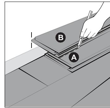
9 To lay the last row: position a loose plank (A) exactly on top of the last row laid. Place another plank (B) on top, with the tongue side touching the wall. Draw a line along the edge of this plank (B), to mark the first plank (A). Cut along this line, plank (A), to obtain the required width. Insert the cut plank against the wall. The last row must be at least 2" wide. The expansion gap spacers can now be removed from the perimeter of the room.
