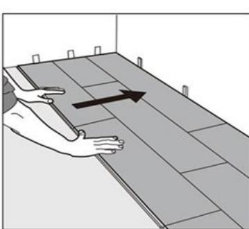
8 After 2-3 rows. Adjust the distance to the front wall by leaving an expansion gap of 1/4". Always ensure that the end joints are staggered at least 8", both when in the same row as when from one row to the next one.
